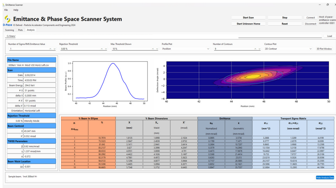
Screenshot of the analysis software presenting results from a scan of a 1 mA, 300 keV H- beam.
